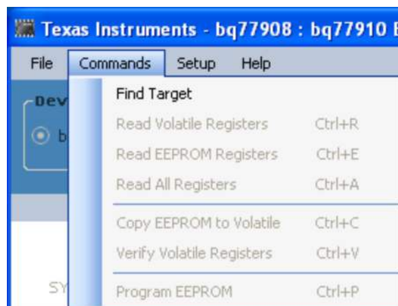
Figure 6. Commands Without Communication Established
