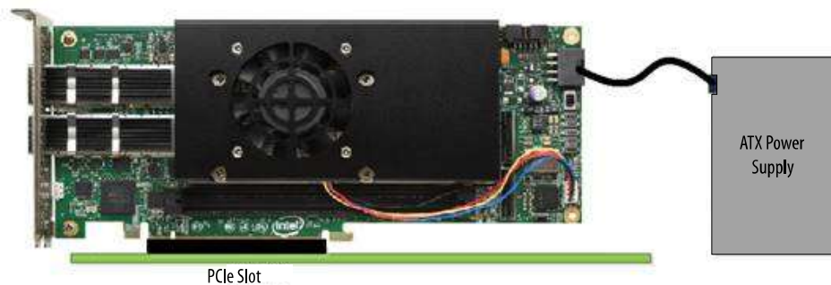
Figure 37. Powering Board Using Standard PCIe-Compliant System
