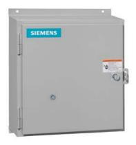
Non-reversing motor starter, Size 2 1/2, Three phase full voltage, Solid-state overload relay, OLRelay amp range 25-100A, 550/575 600 50/60HZ coil, Noncombination type, Enclosure type 12, Dust/drip proof for indoors, Extra-wide enclosure
