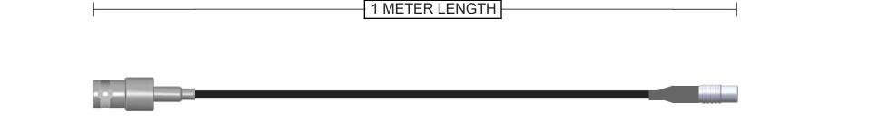
Connector A 112160 BNC Jack Straight Brass Nickel 50 Ohm RG-174 Continuity/Hi-Pot Connector B 252138 MCX Jack Straight Brass Nickel + Heatshrink
