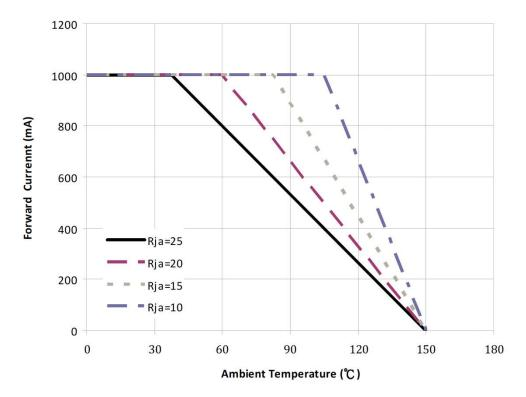
The junction temperature can be correlated to the thermal resistance between the junction and ambient (Rja) by the following equation.
