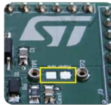
Figure 5. Pads for soldering SMD resistor
