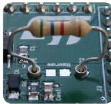
Figure 5. Pads for soldering SMD resistor
