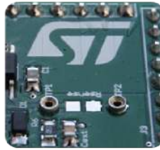
Figure 4. Mounting through-hole sense resistor
