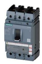
circuit breaker 3VA5 UL frame 250 breaking capacity class M 35kA @ 480 V 3-pole, line protection TM230, FTAM, In=150A overload protection Ir=150A fixed short-circuit protection Ii=5...10 x In UL489 SB (naval), 50 deg. cel. nut keeper kit on both sides
