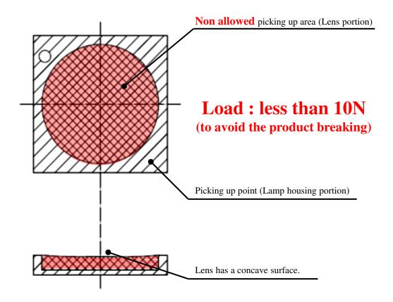
Please adjust the load, the pick up point, the nozzle diameter and etc. before mounting because the over load can cause the breakage of the lamp housing.
