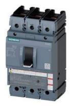
circuit breaker 3VA5 UL frame 250 breaking capacity class H 65kA @ 480 V 3-pole, line protection TM210, FTFM, In=110A overload protection Ir=110A fixed short-circuit protection Ii=10 x In UL489 SB (naval), 50 deg. cel. nut keeper kit on both sides
