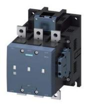
vacuum contactor, AC-3 225 A, 110 kW / 400 V AC (50-60 Hz) / DC operation 200-277 V AC/DC auxiliary contacts 2 NO + 2 NC 3-pole, frame size S10 busbar connections drive: electronic with PLC interface 24 V DC
