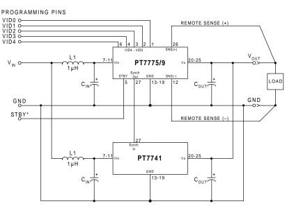
External Capacitors: When used with a PT7779, the PT7741 requires a minimum ouput capacitance of 330µF. The maximum allowable output capacitance is 30,000µF. The PT7741 also requires a minimum input capacitance of 2400µF, which must be rated for a minimum of 2.0Arms of ripple current. For transient or dynamic load applications, additional capacitance may be required. For further information, see the accompanying application note on capacitor selection for this product.
