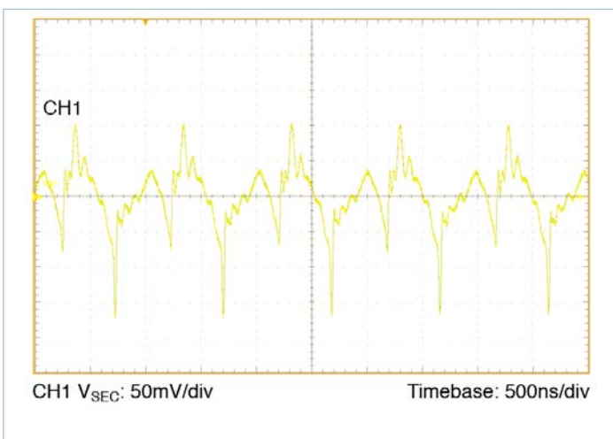
Figure 14 — Full load ripple, 10\mu F C_{PRI\_IN\_EXT} ; No external C_{SEC\_OUT\_EXT} . Board mounted module, scope setting: 20MHz analog BW
