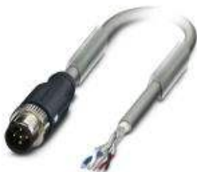
Bus system cable, CANopen®, 5-position, PUR halogen-free, Gray RAL 7001, shielded, Plug straight M12-SPEEDCON, A-coded, on Free cable end, Cable length: 10 m
