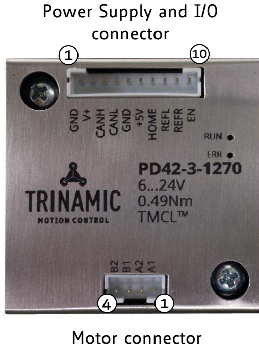
Figure 8: TMCM-1270 connectors
