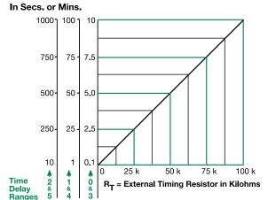
This chart applies to externally adjustable part numbers. The time delay is adjustable over the time delay range selected by varying the resistance across the  $R_T$  terminals; as the resistance increases the tie delay increases.
