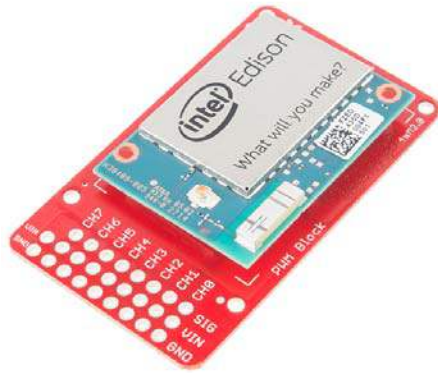
PWM Block Installed
