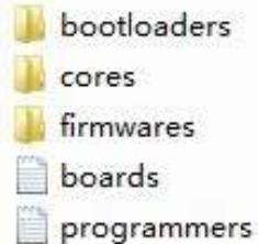
step4: Put the file **boards** of step2 instead of the one **boards** of step3. Then re-open Arduino 0023 and select: **[Optiboot] Lilypad Arduino w/Atmega 168**
