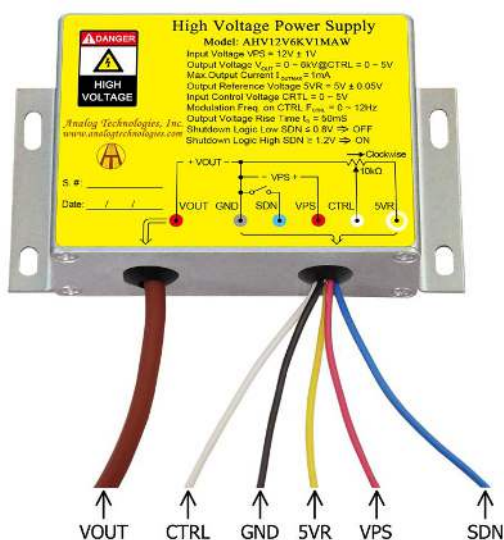
Figure 2. The Connecting Lead Wires of AHV12V6KV1MAW
