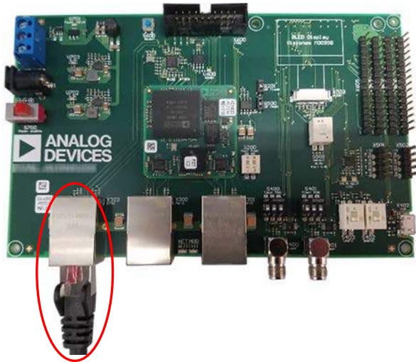
Figure 5. Ethernet Cable Connection
