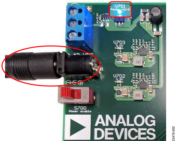
Figure 2. Power Cable Connection and Power Valid LED
