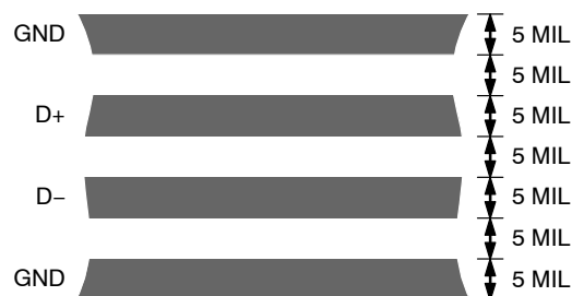
Figure 22. Typical Arrangement of Signal Tracks
