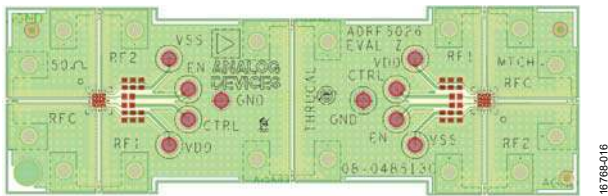
Figure 16. Evaluation Board Layout
