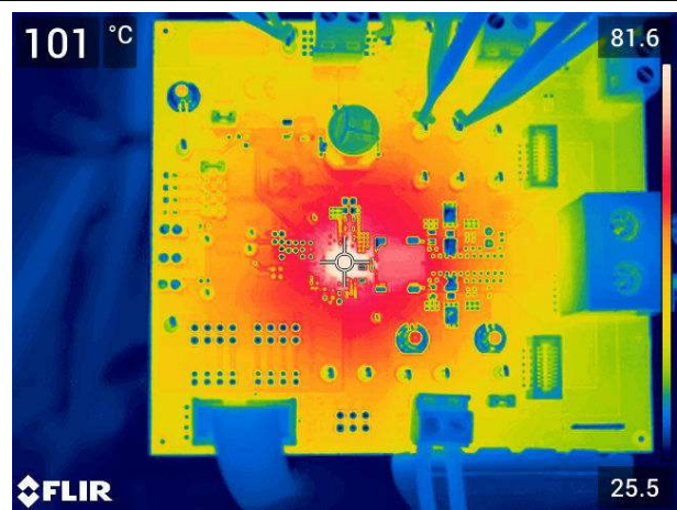
Figure 2-26. Thermal Characteristics, 1.2-MHz FCCM, External 5-V Bias, 35-A Load
