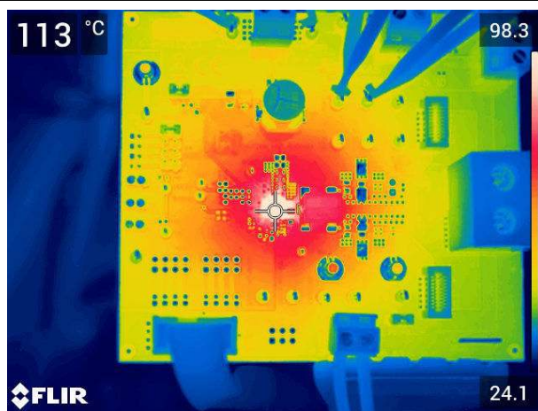
Figure 2-25. Thermal Characteristics, 1.2-MHz FCCM, Internal LDO, 35-A Load
