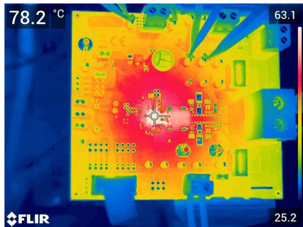
Figure 2-22. Thermal Characteristics, 600-kHz FCCM, External 5-V Bias, 35-A Load
