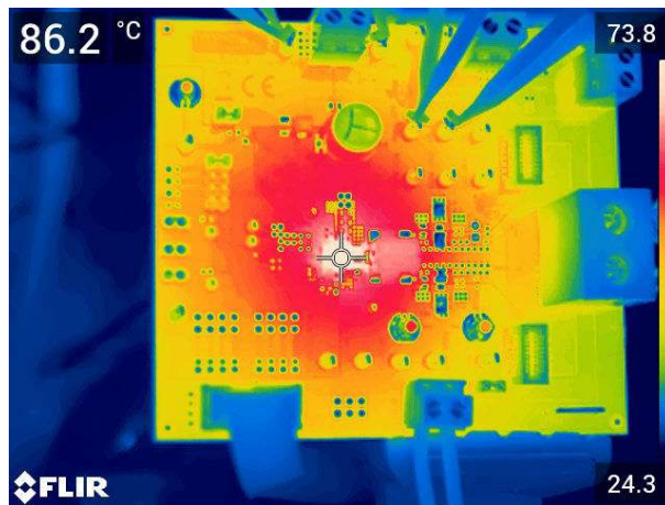
Figure 2-21. Thermal Characteristics, 600-kHz FCCM, Internal LDO, 35-A Load
