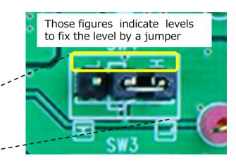
On this evaluation board, jumpers as shown in the picture above are provided for setting operation of TB67S269FTG
