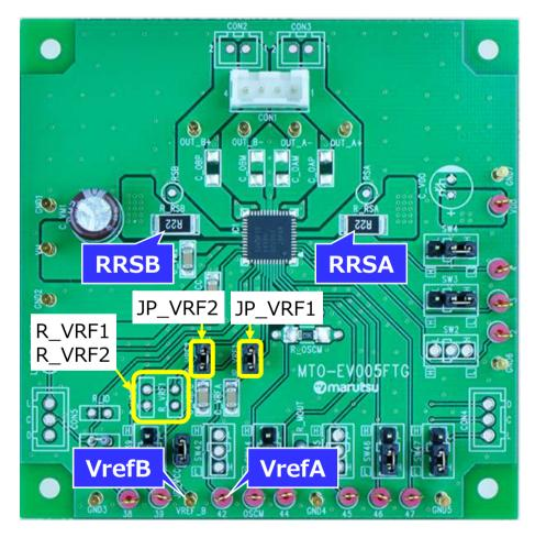
The TB67S269FTG conducts motor operation by PWM constant current control which is based on the frequency of the OSCM oscillation circuit. The maximum current value (set Motor current value) can be determined by a sense resistor (RRS) and the reference voltage (Vref).
