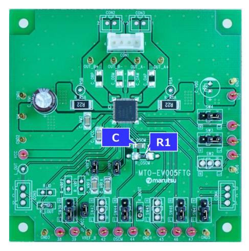
In PWM control of the TB67S269FTG, the internal oscillation frequency (fOSCM) and the chopping frequency (fchop) can be adjusted according to the constant of the external components those are connected to the OSCM pin. In general,  $f_{chop}$  is recommended to set in the frequency range of 50kHz to 100kHz.
