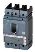
circuit breaker 3VA5 UL frame 250 breaking capacity class H 65kA @ 480V 3-pole, line protection TM230, FTAM, In=100A overload protection Ir=100A fixed short-circuit protection Ii=5...10 x In UL 489 SB (naval), 50° C without connection
