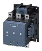
vacuum contactor, AC-3 225 A, 110 kW / 400 V AC (50-60 Hz) / DC operation 575-600 V AC/DC, auxiliary contacts 2 NO + 2 NC, 3-pole, frame size S10, busbar connections drive: conventional
