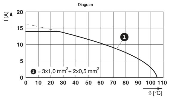
I = current strength, θ = ambient temperature, 3x 14 A + 2x 2 A constant
