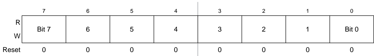
Figure 18-5. Data Direction Register B (DDRB)
