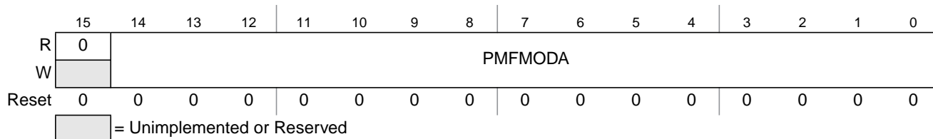
Figure 11-29. PMF Counter Modulo A Register (PMFMODA)
