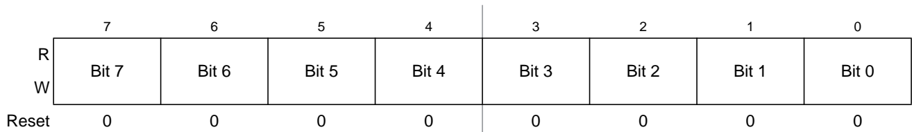
Figure 16-18. Debug Comparator A Register Low (DBGCAL)
