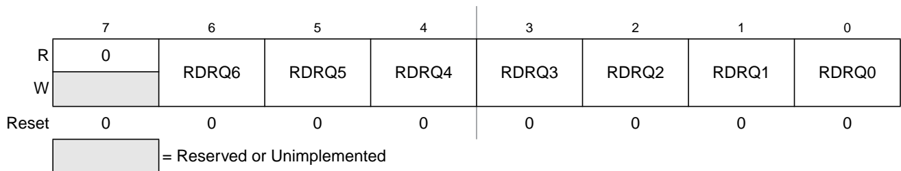
Figure 3-26. Port Q Reduced Drive Register (RDRQ)
