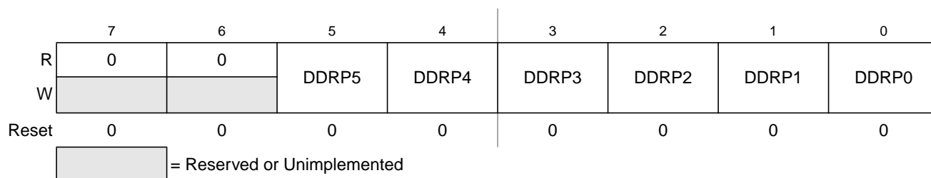
Figure 3-19. Port P Data Direction Register (DDRP)
