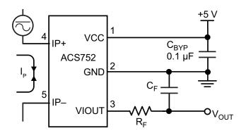
Application 1. The ACS752 outputs an analog signal,  $V_{OUT}$ . that varies linearly with the uni- or bi-directional AC or DC primary sampled current,  $I_{\rm P}$ , within the range specified.  $C_{\rm F}$  is recommended for noise management, with values that depend on the application.
