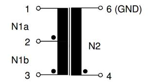
Recommendation: Connect Pin 6 on PCB to GND
