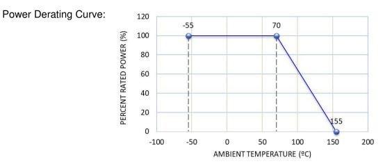
Power rating or current rating is in the case based on continuous full-load at ambient temperature of 70°C. For operation at ambient temperature in excess of 70°C, the load should be derated in accordance with figure of derating curve.
