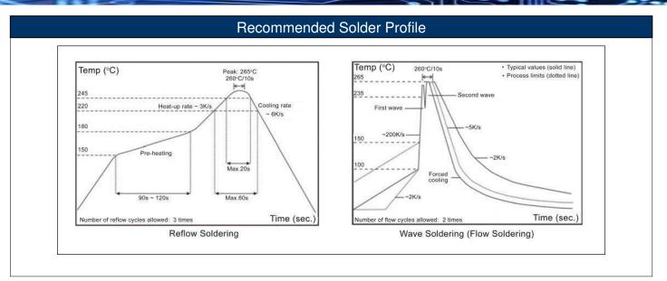
Rework temperature (hot air equipment): 350°C, 3~5 seconds
