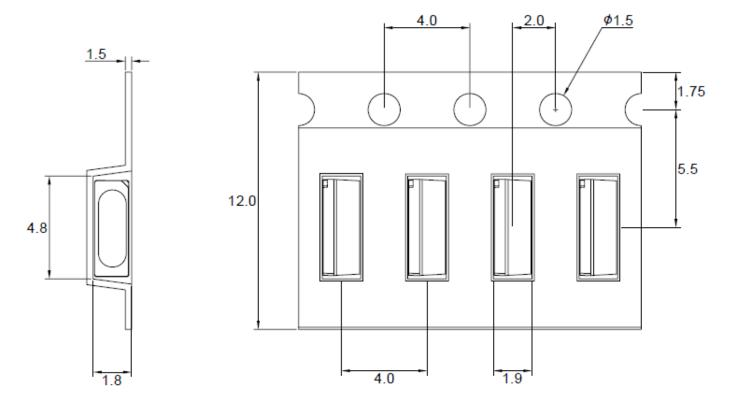
Note : The tolerances unless mentioned is  $\pm 0.1$  mm, Angle $\pm 0.5$ . Unit=mm.
