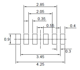
Note : The tolerances unless mentioned is ±0.1mm,Angle±0.5. Unit=mm.
