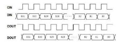
The serial command is transmitted with MSB first, DIN is latched at the rising edge of CIN clock. COUT and DOUT are re-generated for the next RGB LED. COUT is inverted from CIN. When 32 consecutive 0's are encountered, the next 1 is expected to start a 32-bit command, i.e., FLAG[2:0]=111. When FLAG[2:0]=111, then DIMMING, BLUE, GREEN and RED fields are latched respectively.
