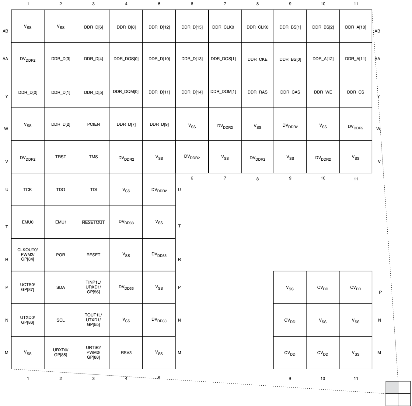
Figure 2-10. ZDU Pin Map [Quadrant A]
