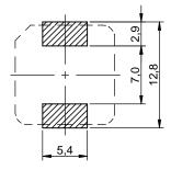
no sensitive traces underneath the component
