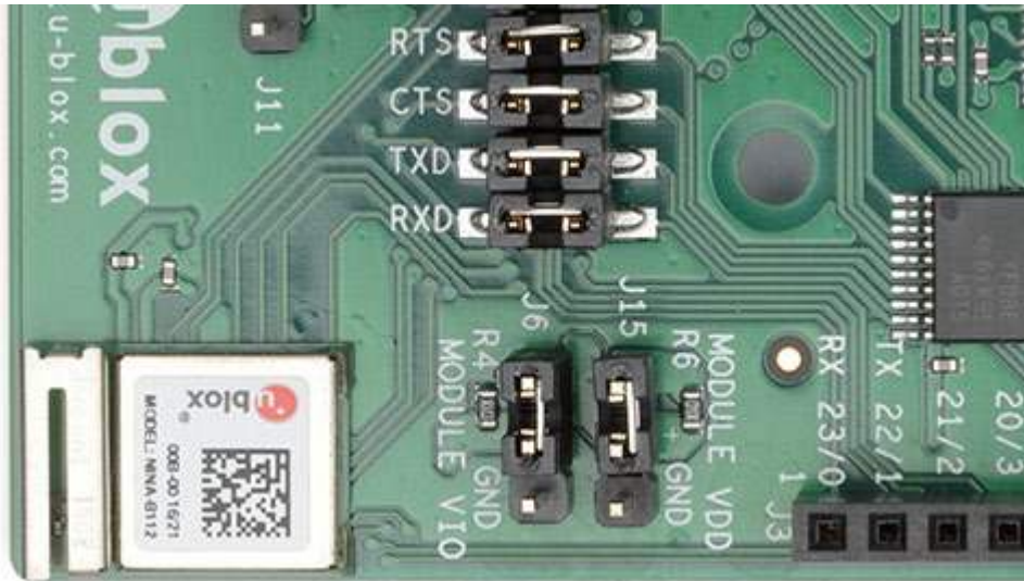
Figure 9: Placement of R4 and R6 (10 \Omega resistors)
