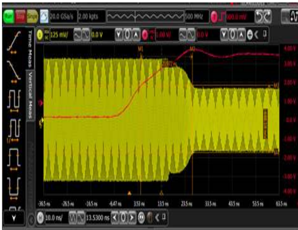
Figure 21. Power OFF Switching Time
