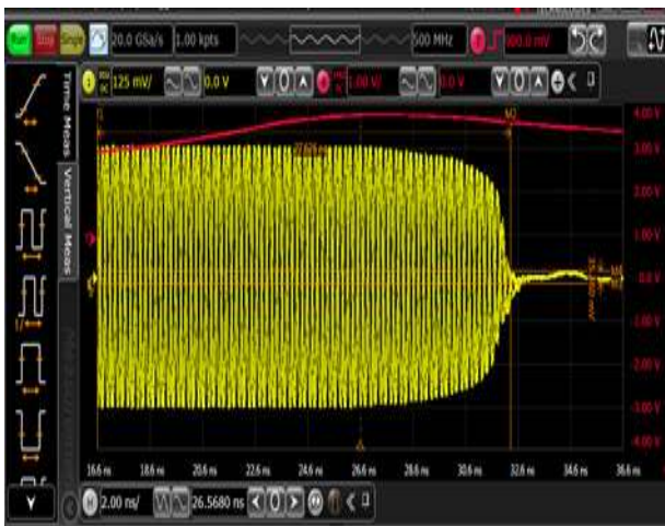
Figure 23. Power OFF to Standby Mode
