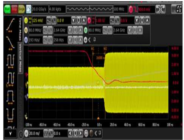
Figure 22. Power ON Switching Time
