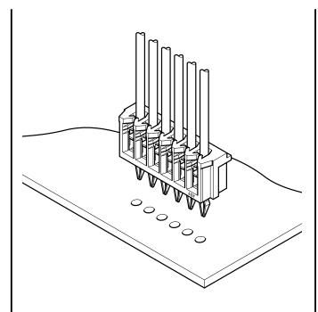
Measuring 2.0mm in pitch, 5.0mm in mounting height, and 4.0mm in thickness, this board-in connector is useful in miniaturizing the connections of small electronic products, such as VCRs, cameras, stereo systems, and car radios. This connector can be used by itself or in combination with the DR connector.
