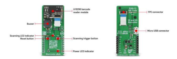
The LV3296 scanner module uses a flat cable to connect to the click board<sup>™</sup>, via the ZIF FPC connector on the back side of the PCB. This flat cable carries all the signals used in communication between the LV3296 module and the host MCU, such as the RX, TX, buzzer, USB, interrupt, reset, and scanning trigger lines.
