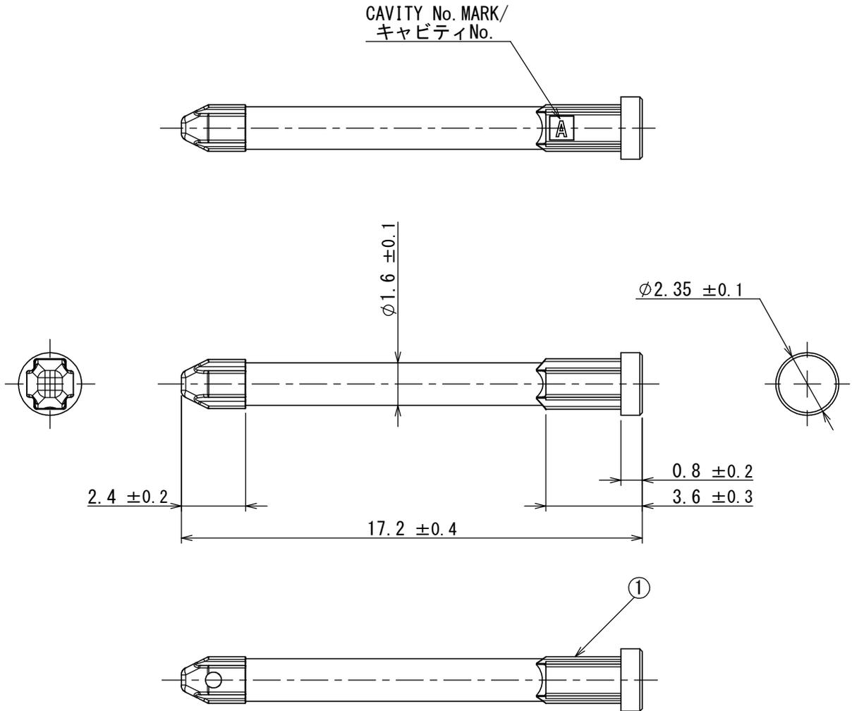
NOTE1. THIS PRODUCT IS DUMMY-PLUG FOR SIGNAL CAVITY OF MX60A SERIES CONNECTOR.
