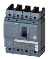
circuit breaker 3VA5 UL frame 250 breaking capacity class H 65kA @ 480V 4-pole, line protection TM230, FTAM, In=100A overload protection Ir=100A fixed short-circuit protection li=5...10 x In N conductor unprotected without connection
