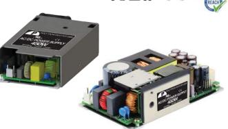
Available in a compact open frame or enclosed package, these 450-watt AC-DC industrial power supplies feature a 5,000-meter operating altitude, 3,000 VAC reinforced insulation and adjustable output voltage.
