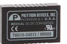
Designed for medical safety and housed in a miniature DIP package, these 10-watt single and dual output DC-DC converters have a patient leakage current of 2 µA and clearance and creepage distance of 8 mm/2 MOPP.
