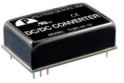
These 5-watt DC-DC converters integrate a six-sided continuous shield and built-in EN55022 Class B filter. Units are housed in an industry-standard DIP package and meet all relevant UL safety standards.
