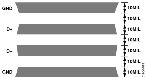
Figure 19. Arrangement of Signal Tracks
