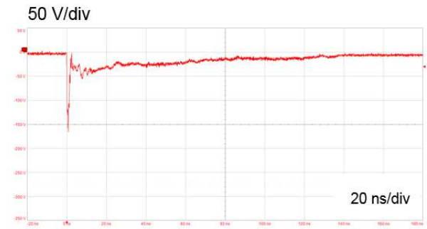
Figure 5. ESD response to ISO10605-C = 150 pF, R = 330 \Omega (-8 kV contact discharge)
