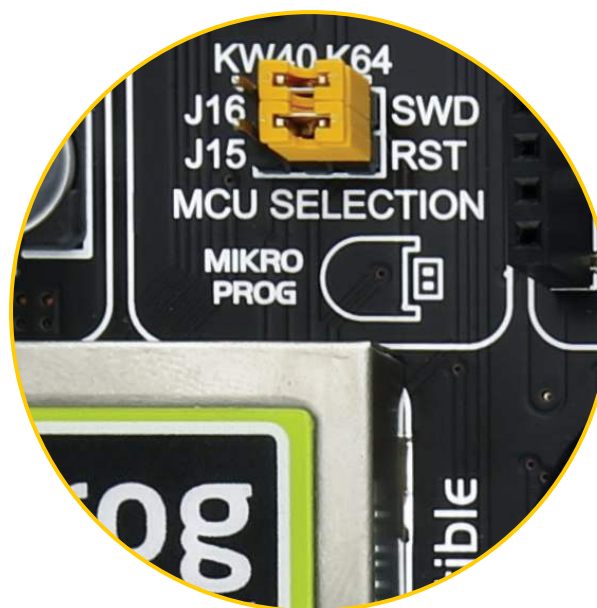
Figure 12: Target MCU selection jumpers
