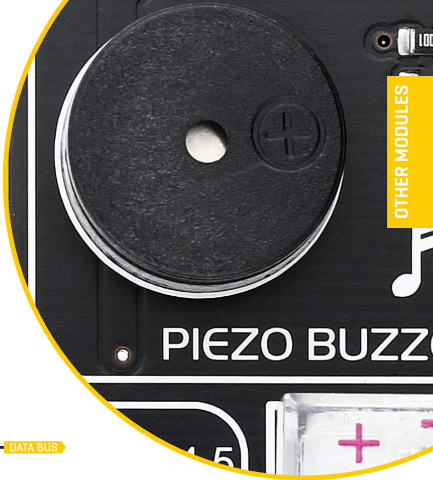
Figure 29: Piezo buzzer with the schematic
