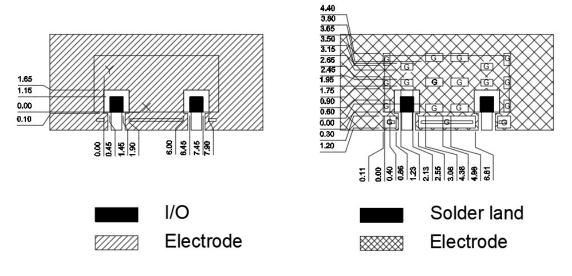
3.6 The recommended shielding case layout guide (min)
