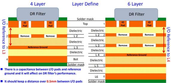
It should keep a distance over 0.5mm between I/O pads and reference ground to avoid large capacitance appear.
