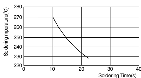
[Allowable Flow Soldering Temperature and Time]
