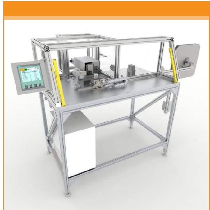
Semi automatic positioning of coil by use of a motor-driven locater unit
