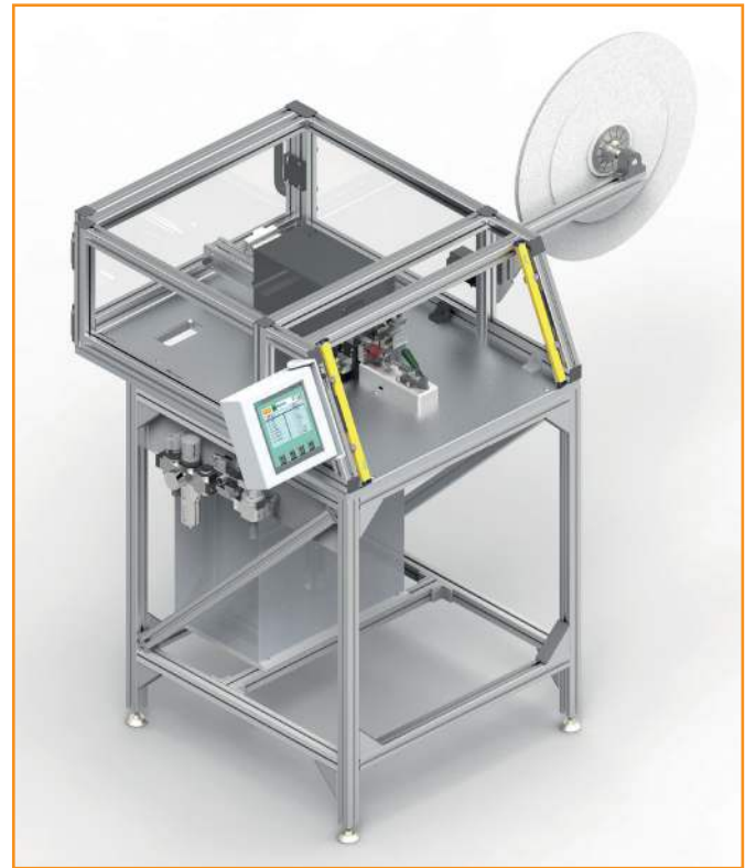
Manual positioning of coil by use of a manually operated locater unit
