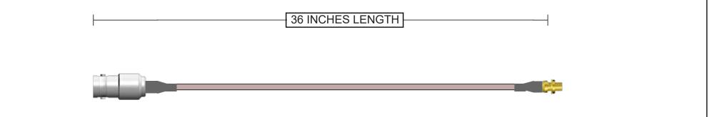
Connector A 112631 BNC Jack Straight Brass Nickel + Heatshrink 50 Ohm RG-178 Continuity/Hi-Pot Connector B 252167 MCX Jack Straight Bulkhead - Rear Mount Brass Gold + Heatshrink
