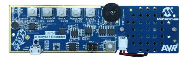
AVR Parrot board implements a voice recorder with ATtiny817. Voice is captured by ADC of ATtiny817 via a microphone, and played back using DAC of ATtiny817. A dataflash device is used to store the acquired voice data.
