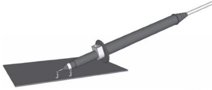
Figure 7. Measuring Input or Output Ripple
