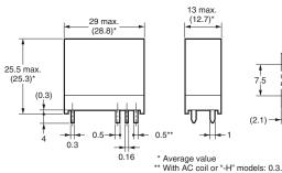
**PCB Mounting Holes** (BOTTOM VIEW) Tolerance: ±0.1 mm
