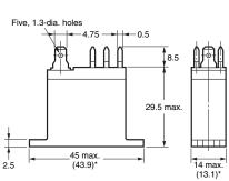
**Mounting Holes** (BOTTOM VIEW) Tolerance: ±0.1 mm
