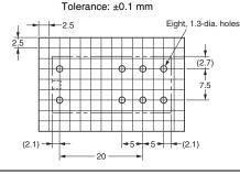
**Terminal Arrangement/** Internal Connections (BOTTOM VIEW)
